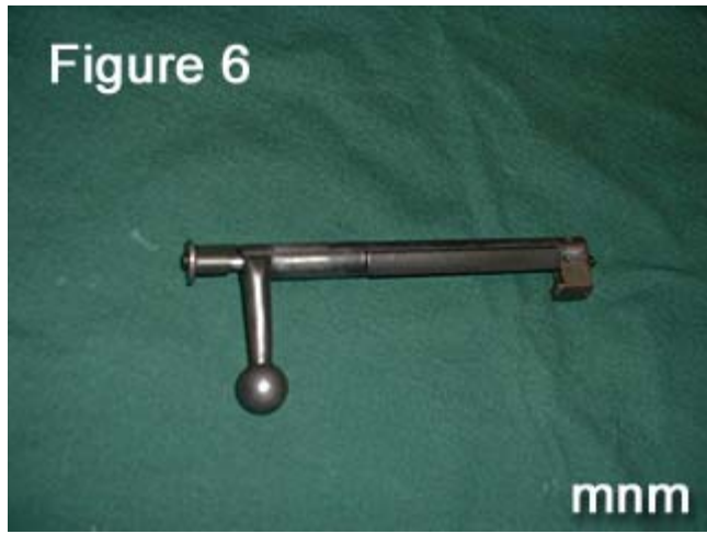
6) Wipe and clean external surface of bolt assembly.
