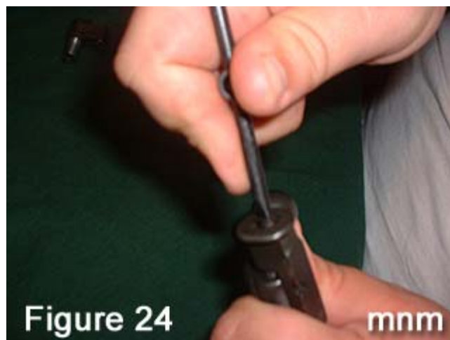
6) Use bolt assembly tool to tighten striker screw.
