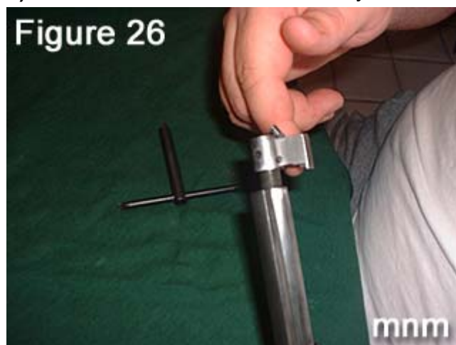
8) Tighten bolt head on threads by rotating it clockwise.
