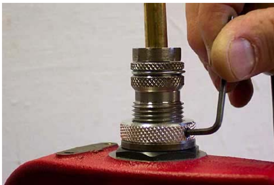
Swaging the primer pocket. Adjustments not finalized yet.
