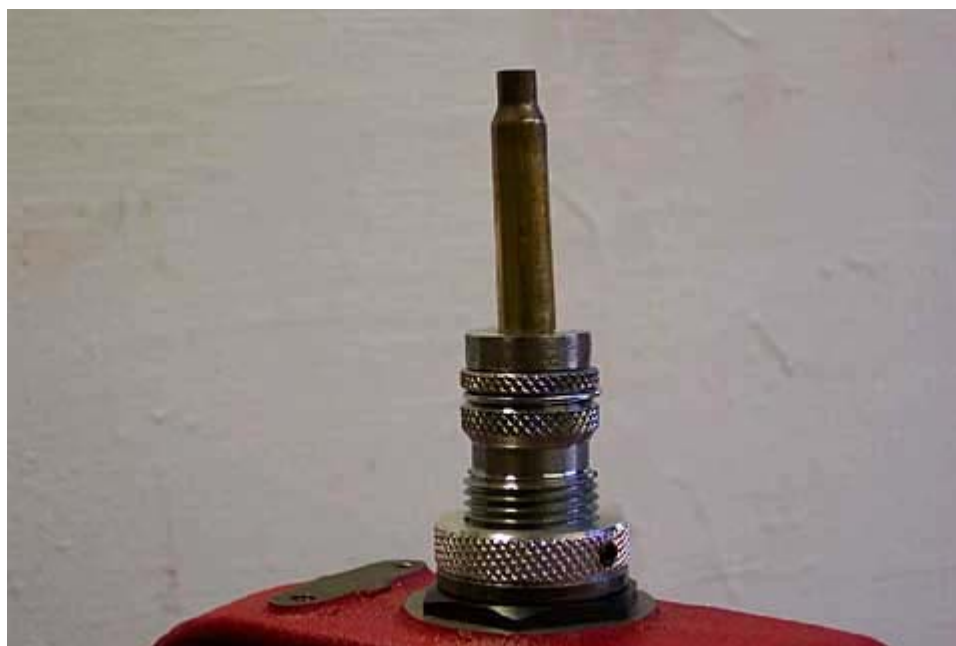
Swaging the primer pocket. Adjustments not finalized yet.
