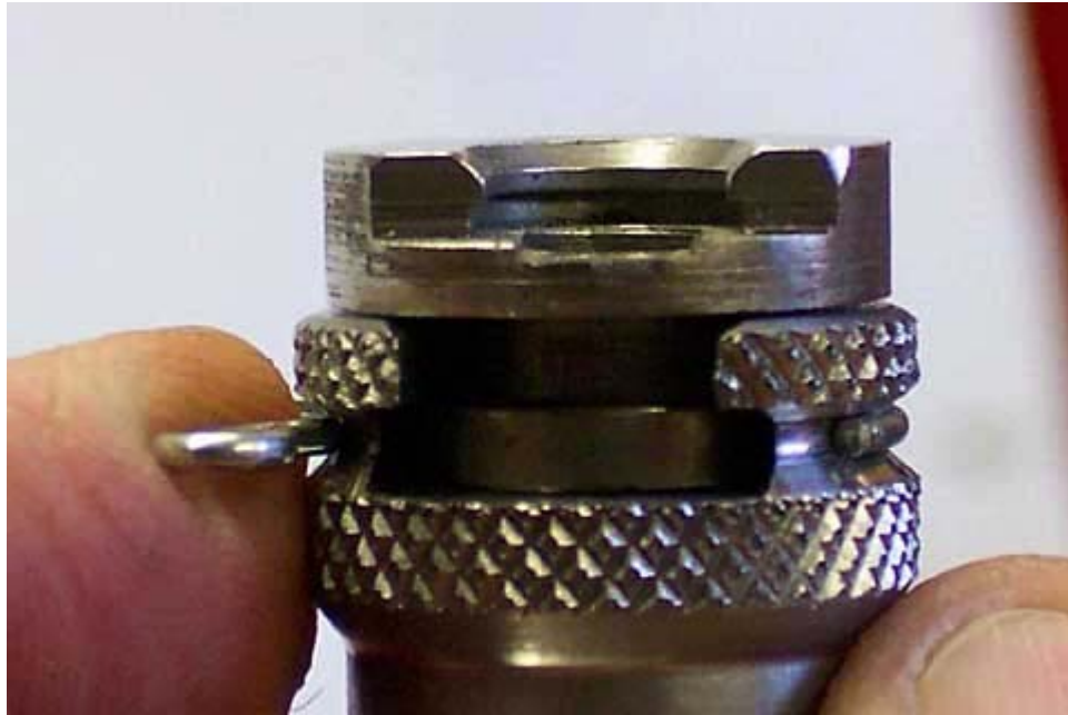
Starting to push finger piece of shellholder-retaining ring.
