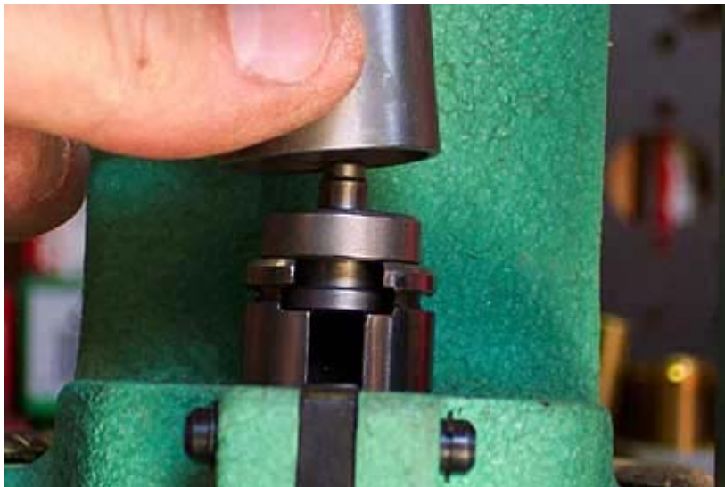
Release cup being slid into place (spring clip is now removed)
