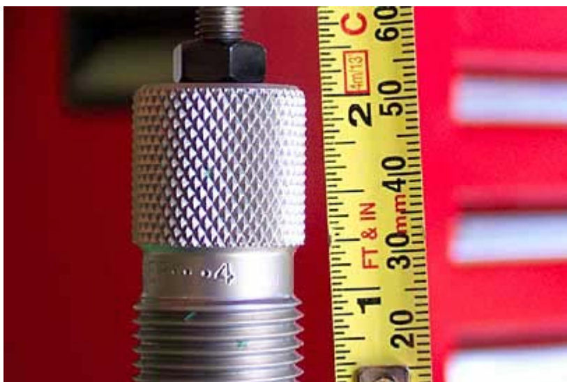
With ram raised to full height, die body is threaded into press until it touches top of release cup.
