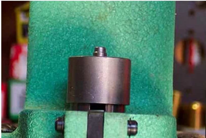
Release cup fully seated, primer punch protrudes
