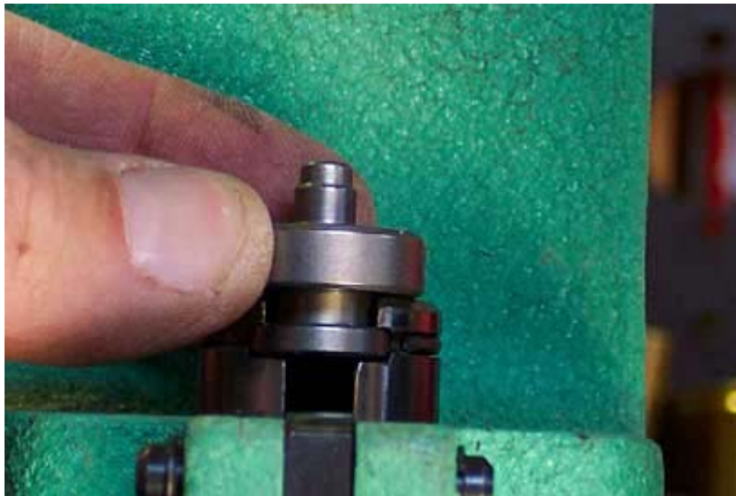
Swager punch being snapped into place (spring clip is still in place)
