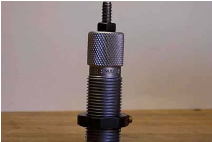
Swager die body with swager rod & rod lock nut installed
