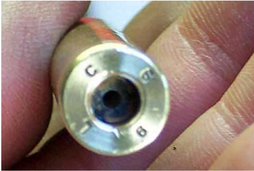
Pocket is correctly swaged
