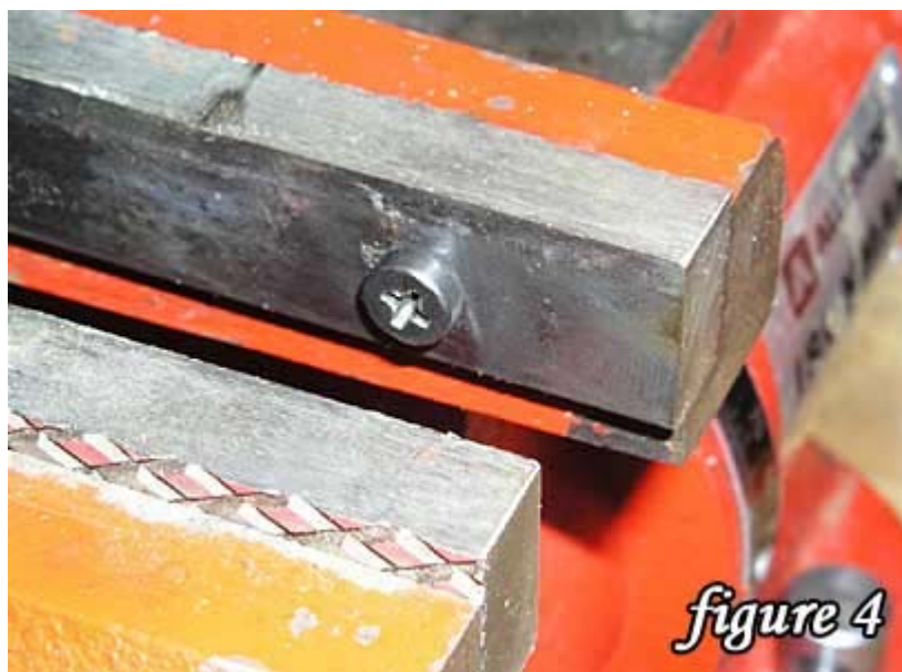
Figure 4. Smooth jaws can be obtained by flipping the vise jaws. Protruding screws do not matter in this case.
