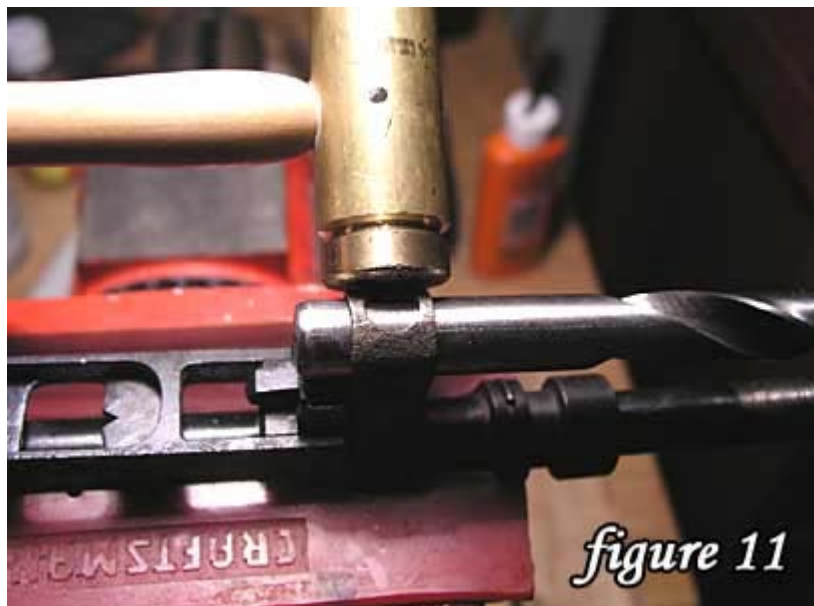
Figure 11. Using brass hammer, pound the front sight hood evenly. Start with light tapping and progressively increase the force of hit until you feel metal is being bent. Reduce the force when tapping near the edges.
