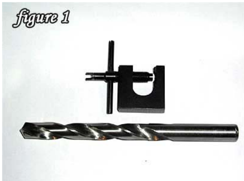
Figure 1. Tools needed to fix the smashed front sight hood, 14mm drill bit and C-tool.
