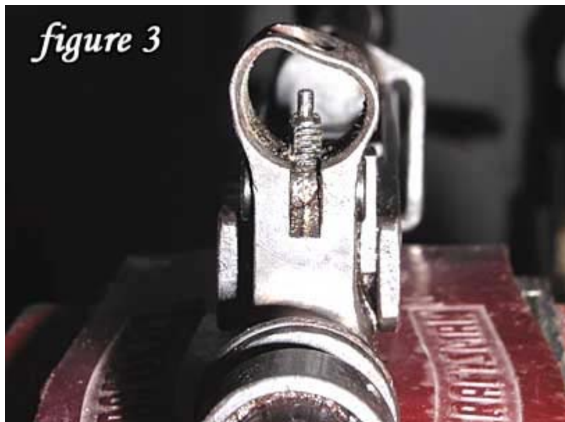
Figure 3. A typical problem with an SKS rifle - a bent front sight hood.
