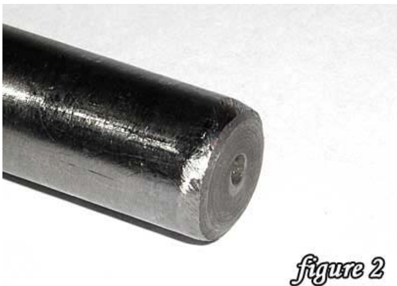
Figure 2. The edge on the shank end of the drill bit is ground off to make it tapered.
