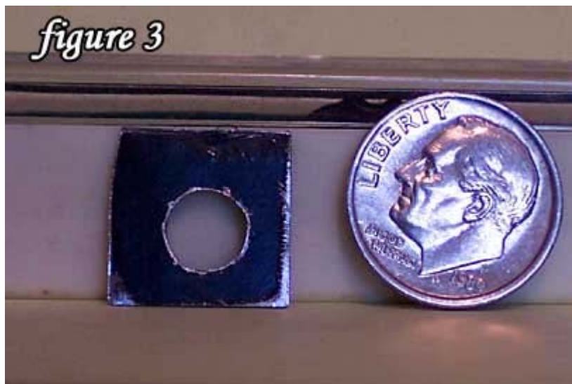
Thin sheet steel, 0.026 cuts easily with tin snips.
