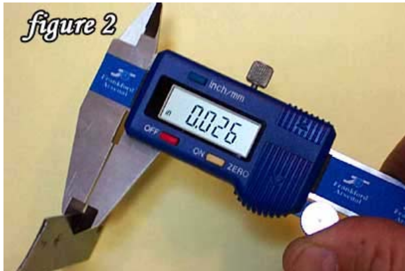
Thin sheet steel, 0.026 cuts easily with tin snips.
