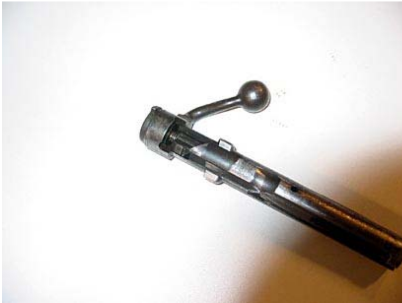
Look at those locking lugs! That is one heavy smooth bolt.
