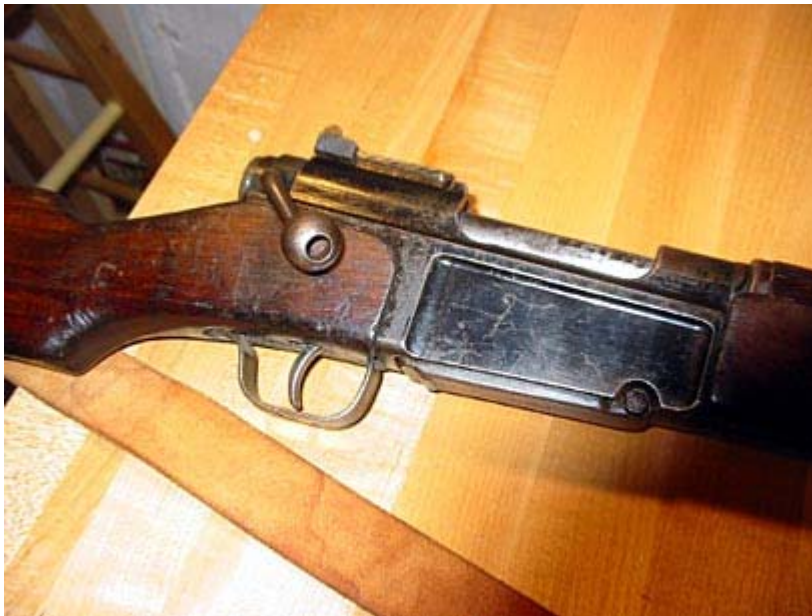
Side view of the MAS 36. Note the baked enamel type finish. Very sturdy and weather resistant, but does scratch! Others will be parkerized various shades of grey.
