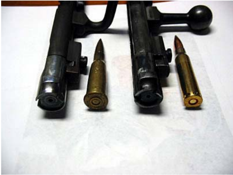
The old Lebel bolt head and the new for the 7.5. Note difference in size!
