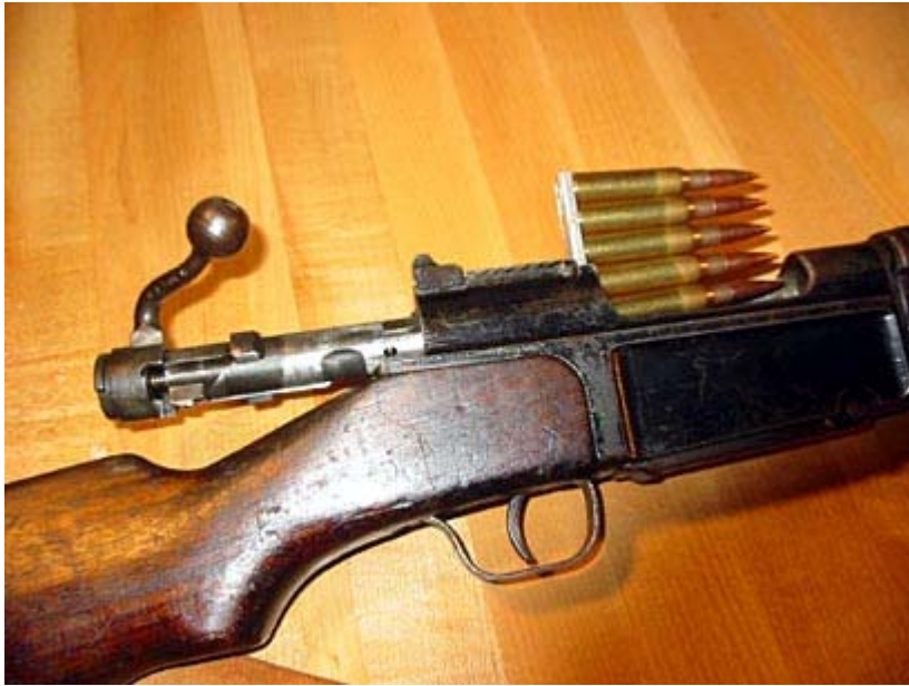
Ready for loading using the uniquely French stripper clip. Big thumb cut out on the other side helps.
