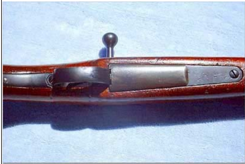
The bottom of the weapon showing the magazine floor plate
