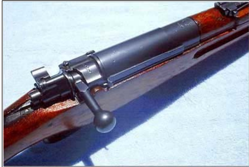
The receiver shown with the sliding dust cover in the closed position
