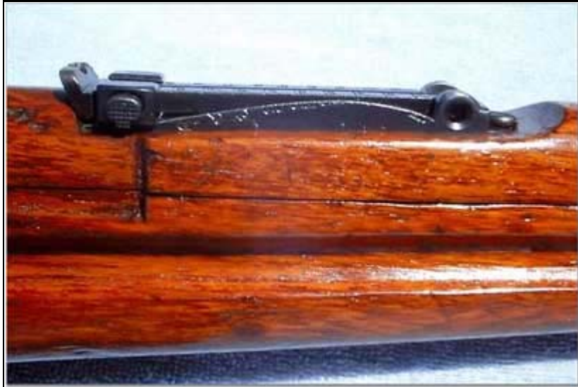
The rear sight base, notice this one has been cut down for the 8x52Rmm Type 66 cartridge
