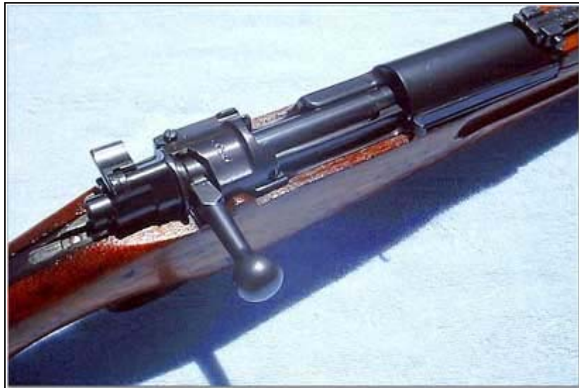
The receiver shown with the sliding dust cover in the open position
