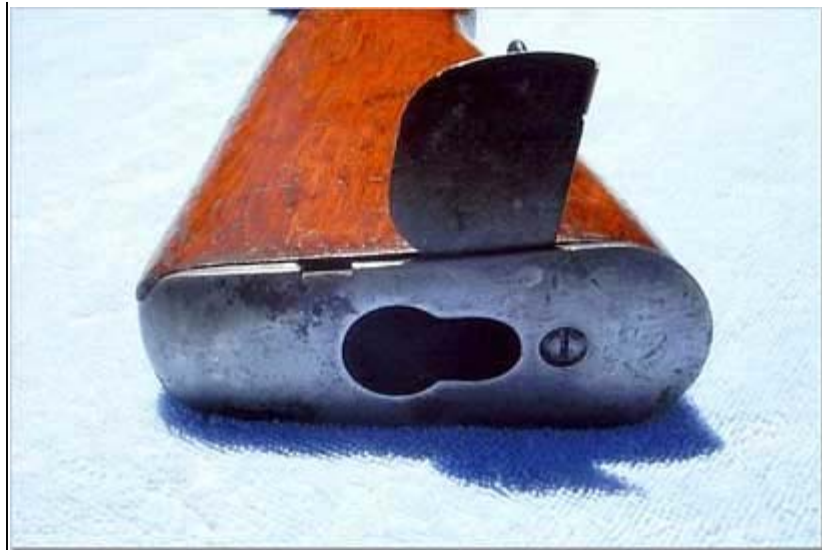
The sliding cover plate on the buttplate in the opened position
