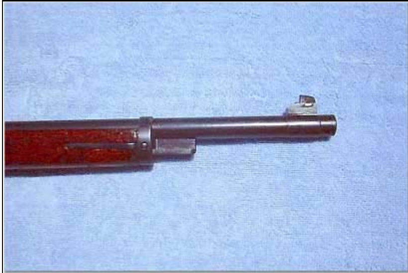
The front sight, front barrel band and the bayonet lug What is missing is the cleaning rod
