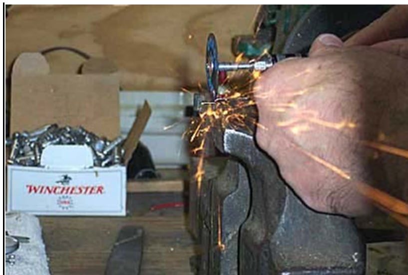
Excess pin is clamped in the vice, Dremel tool cuts it off
