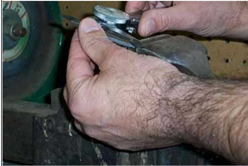
Determining center of sight base with a caliper
