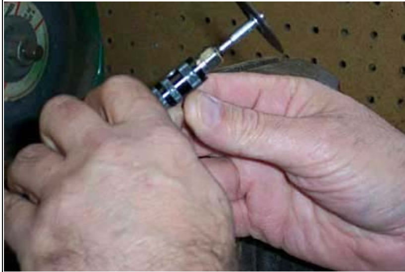
Use Dremel Tool to remove blade from front sight
