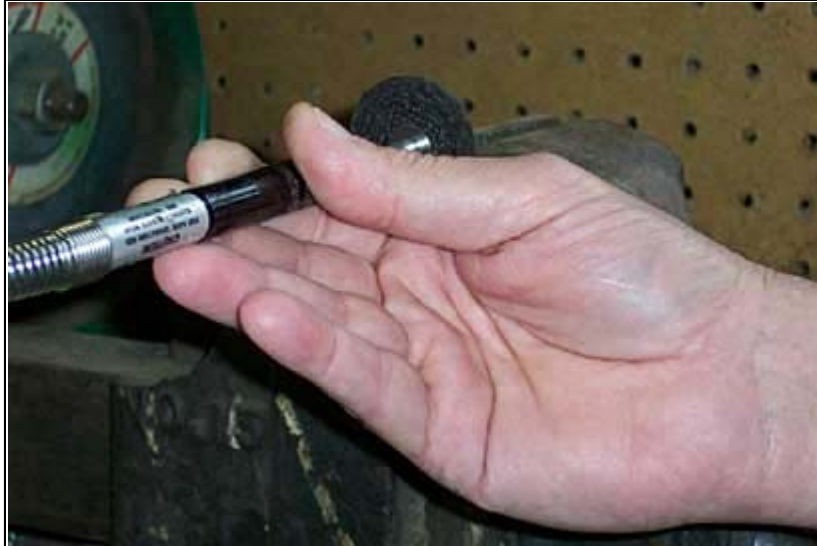
Impregnated cut-off wheel and a flex shaft make it easy to remove blade while sight base is clamped in a vice
