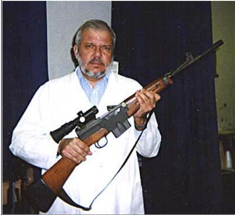
9. The next version, the 49/56 equipped with the 'scope. It's basically a copy of the ZF-4 with the same egregious optics. How the scope and the rifle got married is another saga in the life of a Gun Collector.
