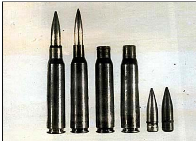
10. The photo shows an unfired 7.5 x 54 mm and a 6.5 x 55 mm Swede, note how similar they are. Next a fired 7.5 and a
