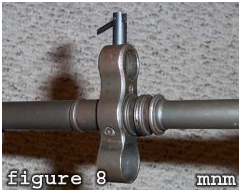
Use of the TAPCO.COM CETME front sight adjustment tool.
