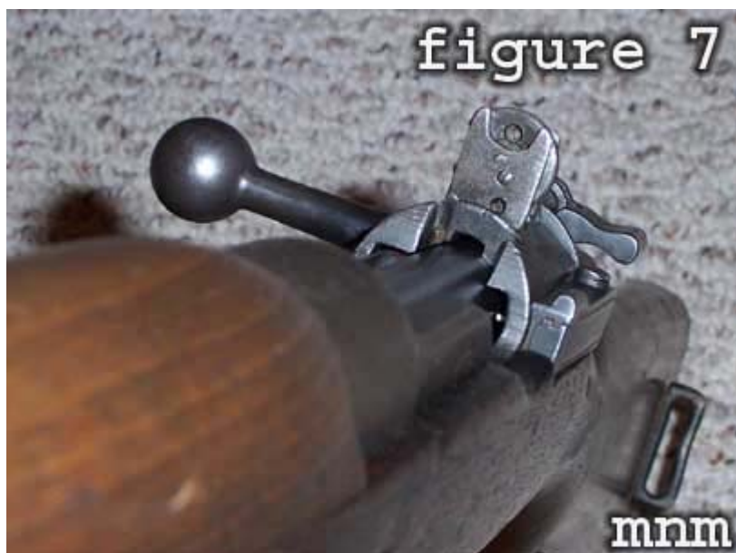
Looking toward the back end of the rifle, note the dial peep rear sight. Also, note the side mounted sling attachment.
