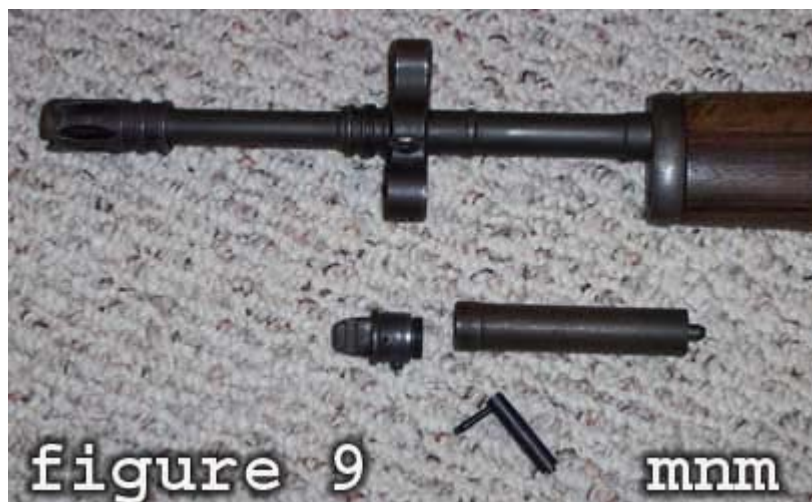
Taking apart the “fake” gas cylinder reveals a clever place to store a cleaning kit, or, in this case, the front sight adjustment tool.
