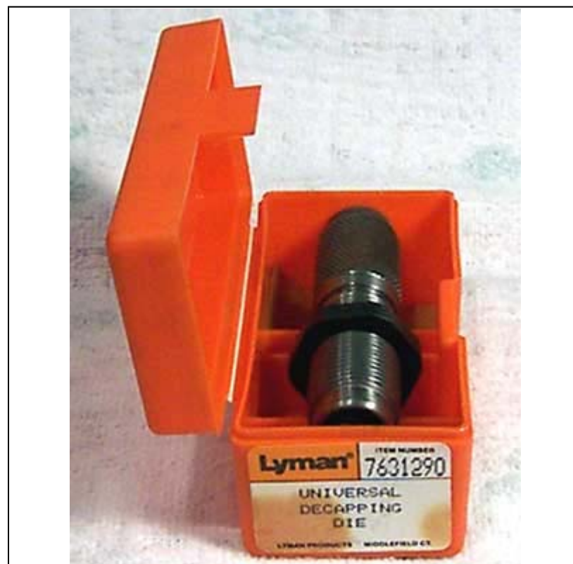
Figure 3. A Lyman Universal decapping die, a very useful item for removing primers (crimped or not) without resizing the brass case. No lube is needed.
