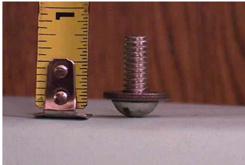
1/4-20 round head bolt and flat washer used in drill press to expand gas checks.
