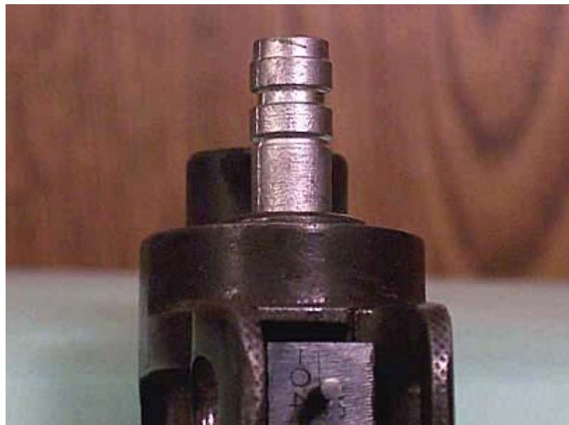
Nose of Saeco .30 cal bullet now fits lands correctly.
