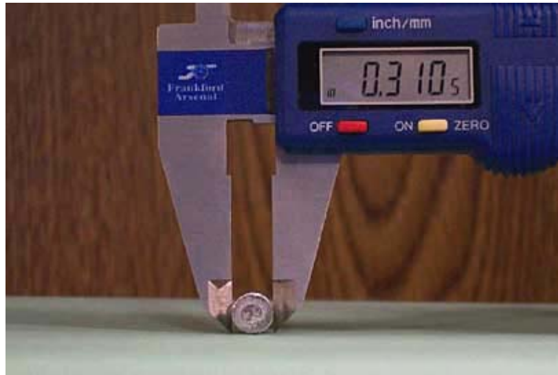
Body of Saeco .30 cal bullet measures 0.3105, this is too small for SMLE grooves.
