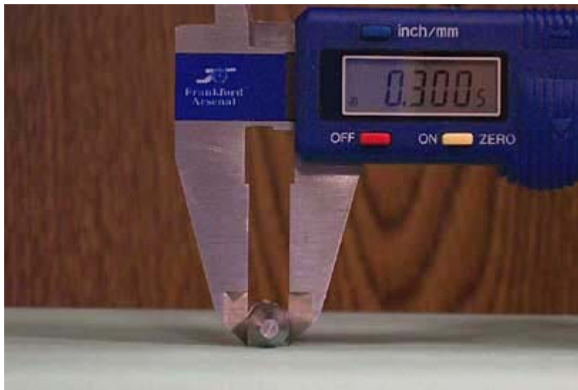
Nose of Saeco .30 cal bullet measures 0.3005, too small for SMLE lands. No wonder it dropped right down muzzle!
