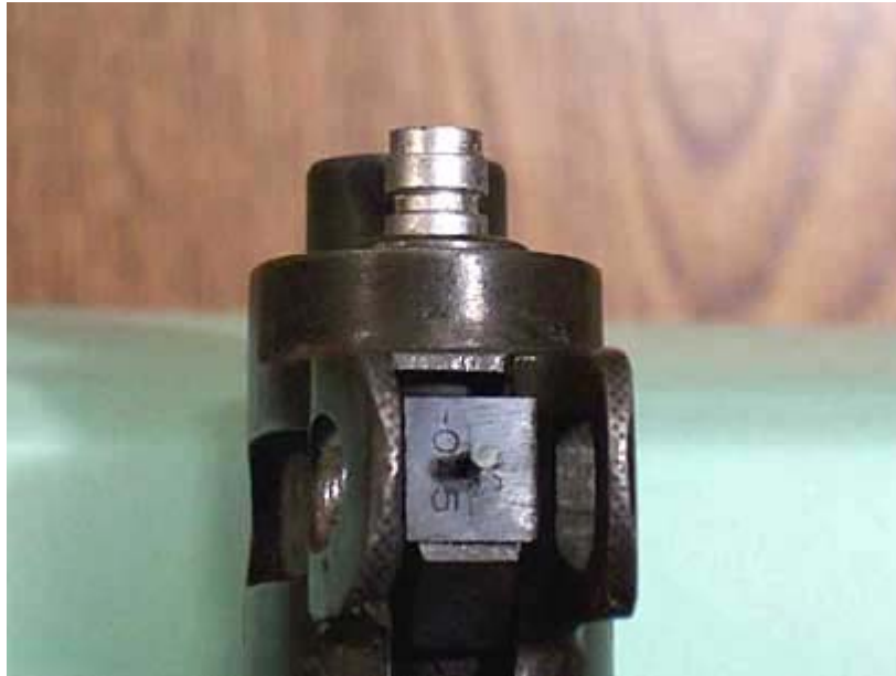
Nose of Saeco .30 cal bullet drops into muzzle of SMLE. This fit is too loose to be accurate!
