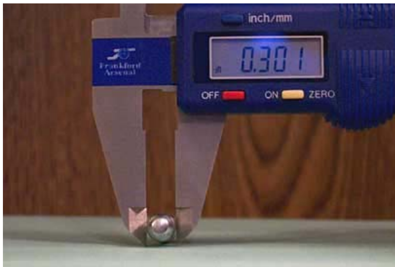
Nose of NEI .30 cal bullet measures 0.301, it will not be supported by SMLE lands.
