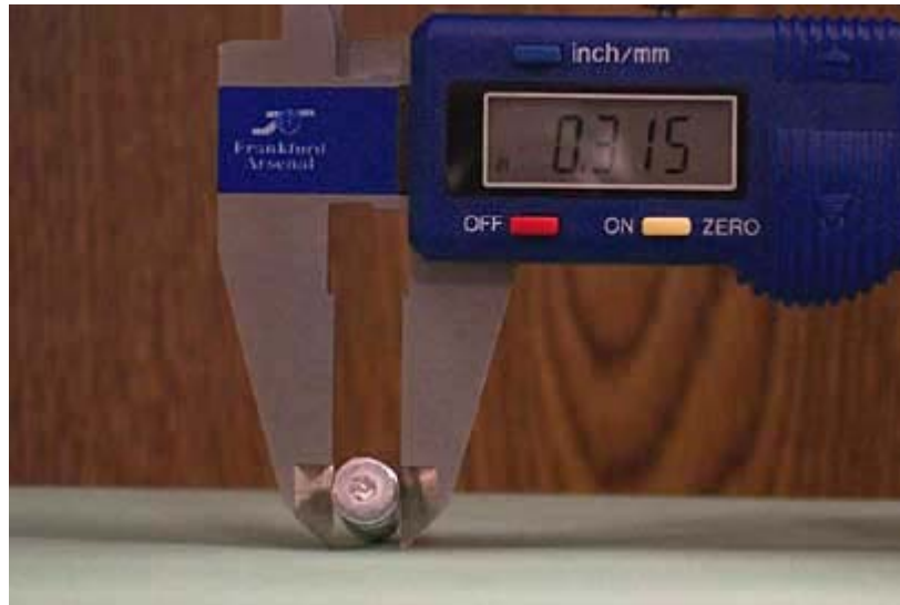
After mould is taped, body of NEI .30 cal bullet now measures 0.315, correct for SMLE grooves.
