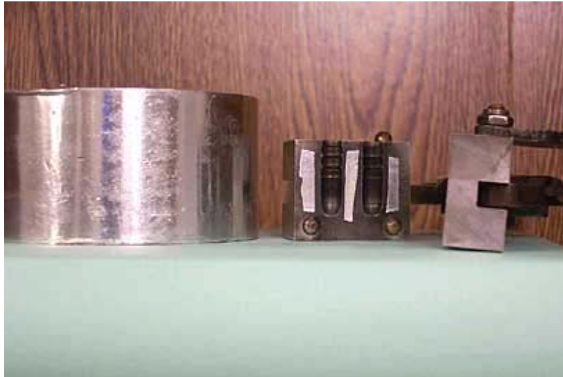
Aluminum duct tape, NIE 180308GC mould, aluminum tape is on both sides of mould.
