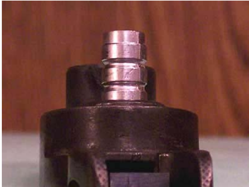
Nose of NEI .30 cal bullet drops into muzzle of SMLE. This fit is also too loose to be accurate!
