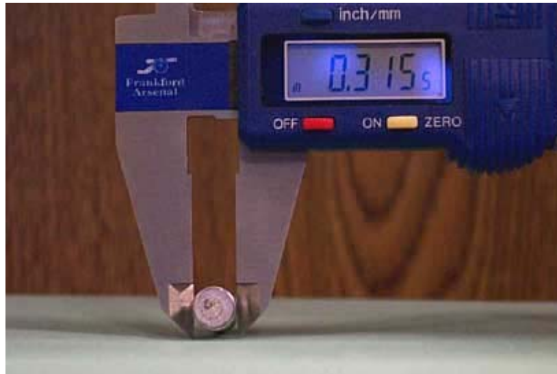
After mould is taped, body of Saeco .30 cal bullet now measures 0.3155, correct for SMLE grooves (bullet still didn't group well though).
