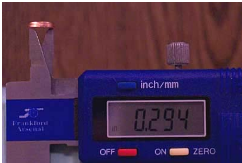
Expanded gas check, plenty of room to correctly seat on large bullet.
