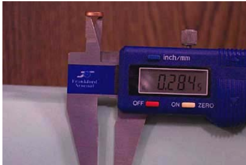
Interior of standard size gas check.
