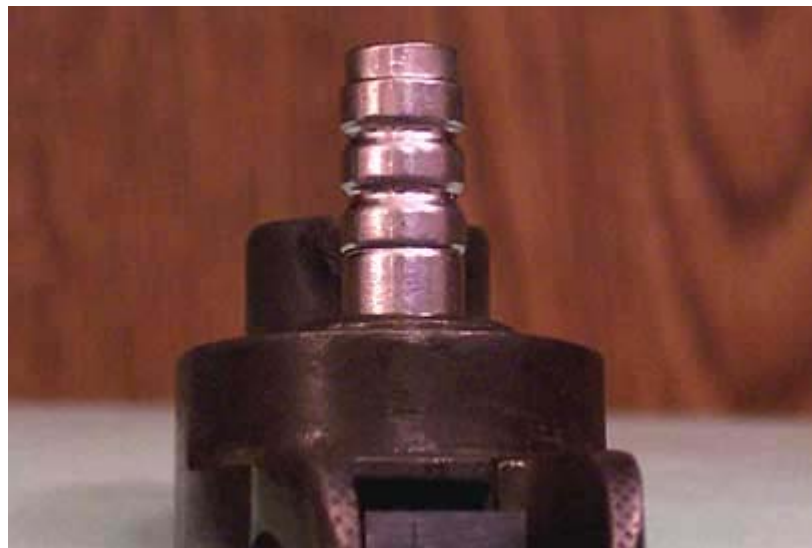
Nose of NEI .30 cal bullet now fits lands correctly. This bullet was successful!
