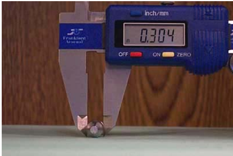
After mould is taped, nose of Saeco .30 cal bullet now measures 0.304, correct for SMLE lands.
