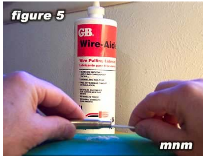
Lubing the Inside of Case with GB using a Cotton Tipped Swab
