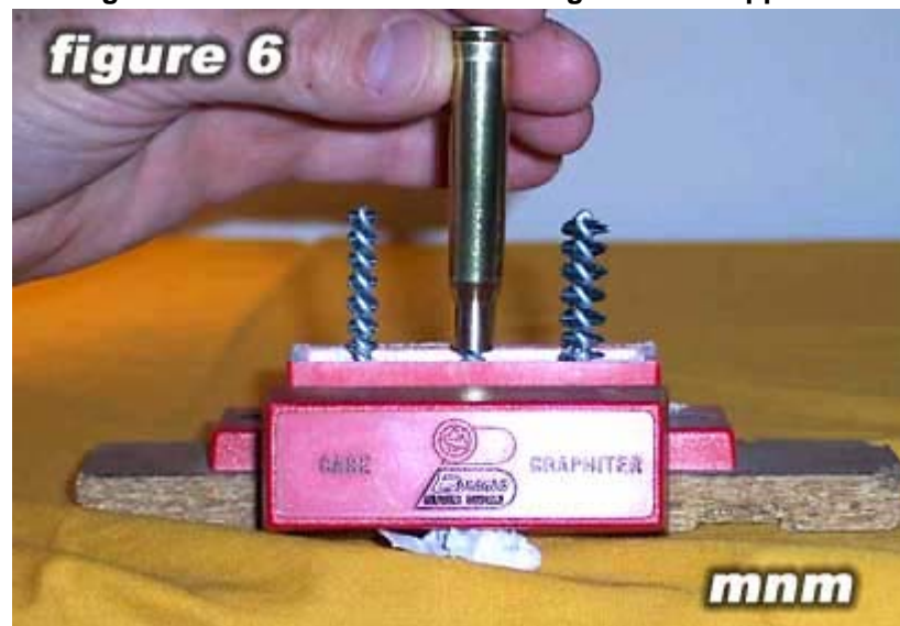
Lubing the Inside of Case with GB using a Cotton Tipped Swab
