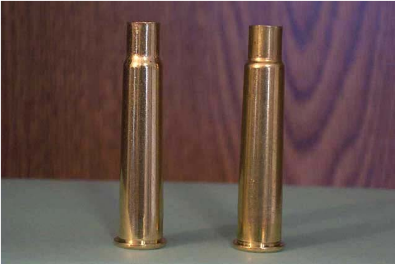
Fig II Unfired Winchester brass & fired Winchester brass. Winchester factory shoulder shape is closer to chamber shape than PMC. But, there is still quite a bit of space between the shoulder and the chamber.
