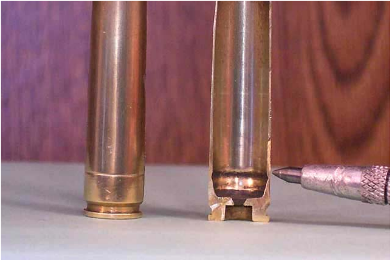
Fig VI Notice groove on inside of bad case at right.
