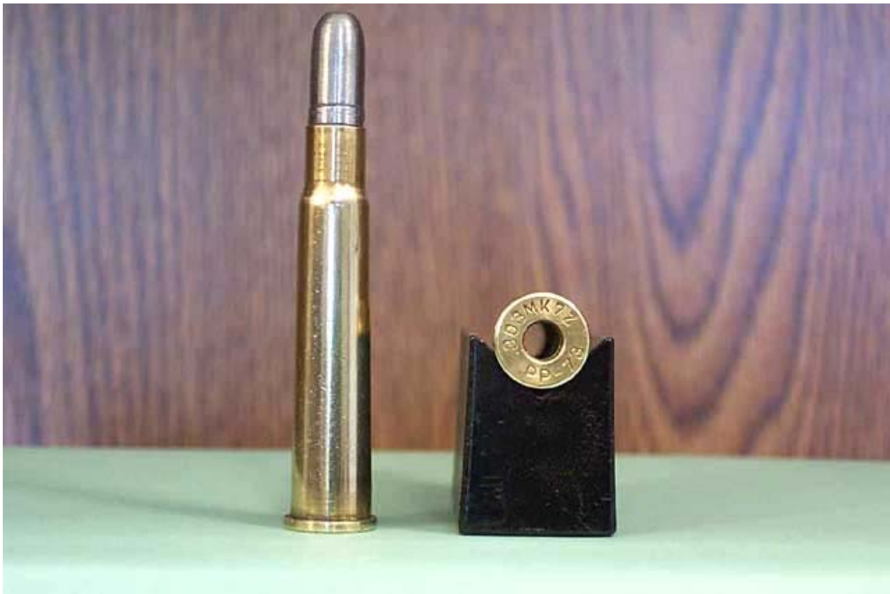
Fig IV Dummy round & primer pocket drilled completely through.
