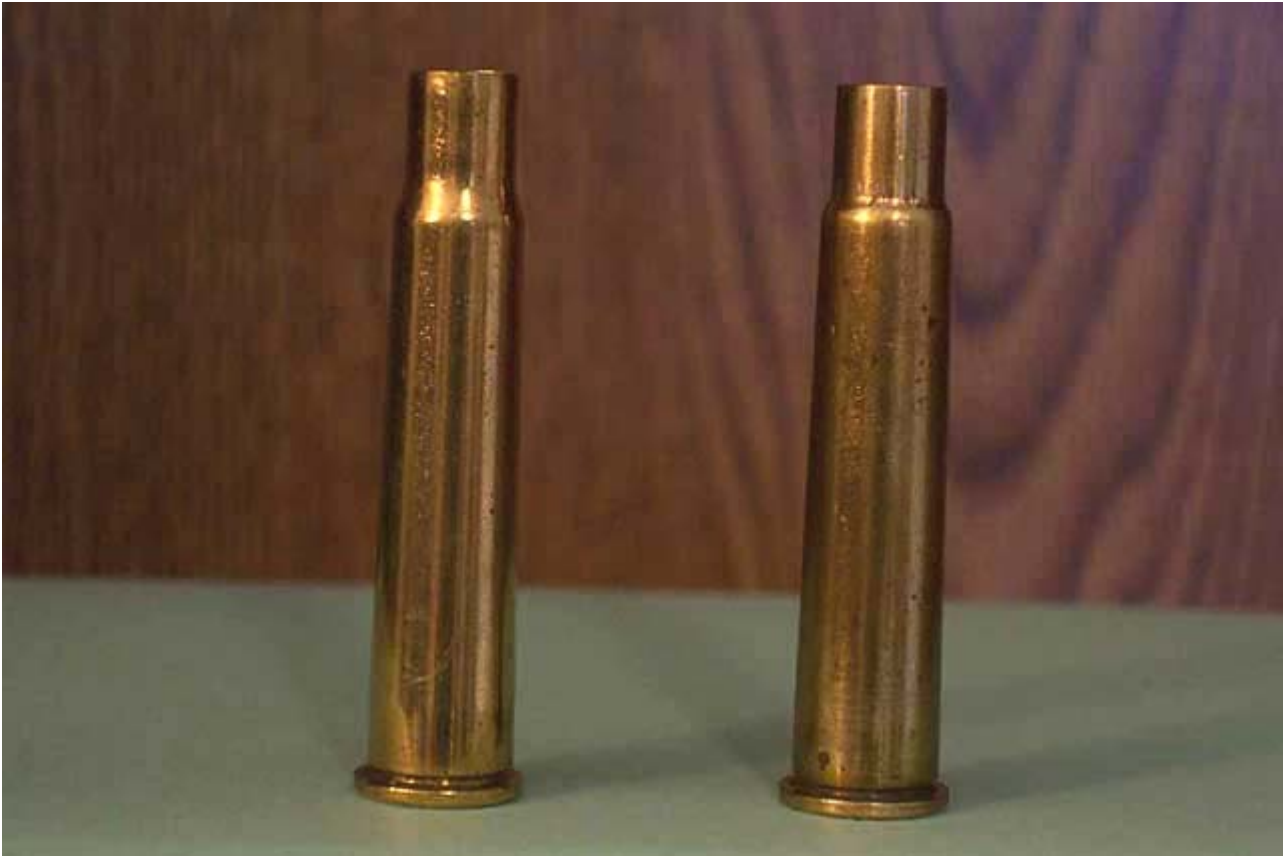
Fig 1 Unfired PMC brass & fired PMC brass. Notice the factory shoulder shape bears little resemblance to the fired cases shoulder.
