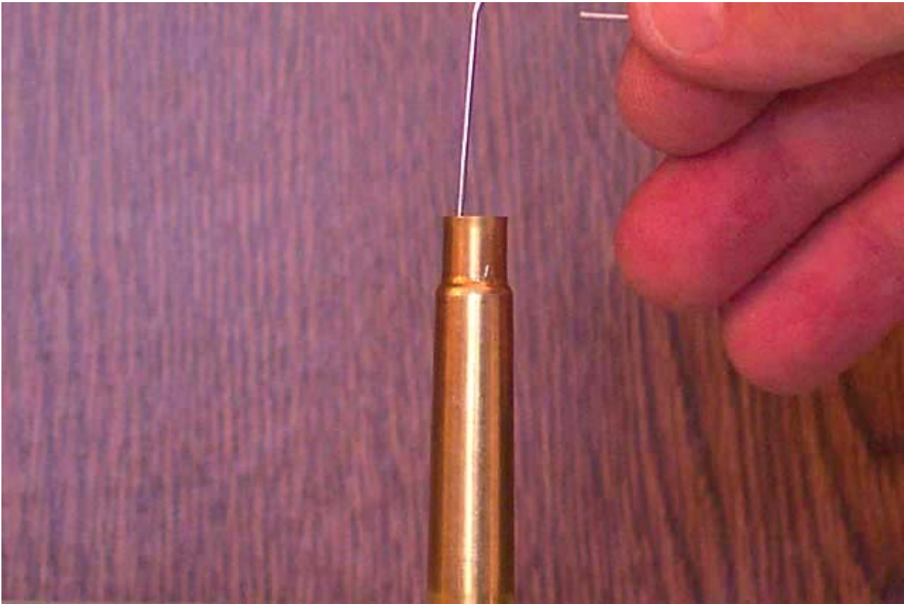
Fig VIII Checking brass for evidence of thin groove.
