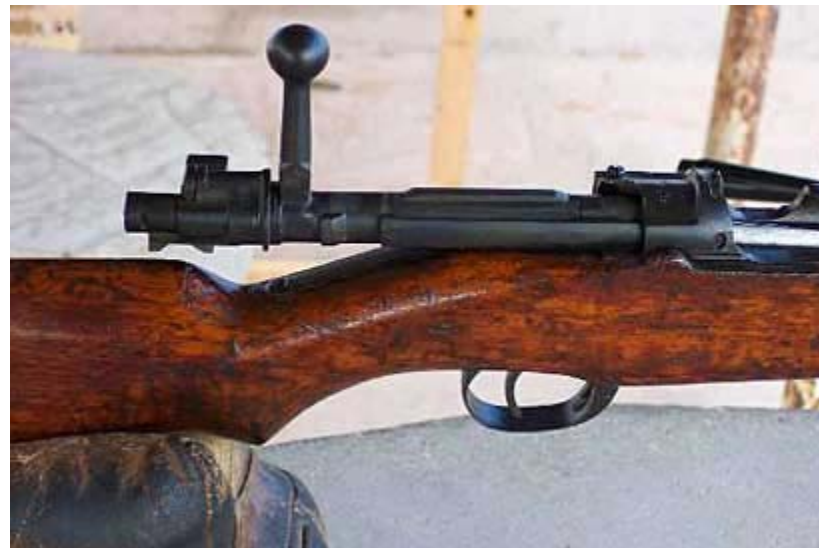
Siamese Mauser, Note Original Safety & Straight Bolt Handle
