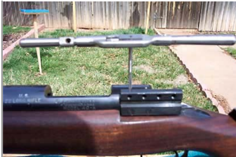
Cleaning Threaded Holes In Receiver.
