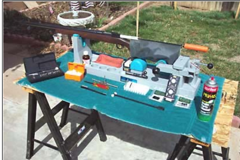
Gunsmith Screwdriver Set, Cleaning Patches, Solvent, Tap & Tap Handle, Bore Brushes, Acton Cleaning Tool, Brush, Bases & Rings, Spray Solvent, Bore Guide With Solvent Port (Inserted In Action), Stock Protector, Bore Tech Cleaning Rod
