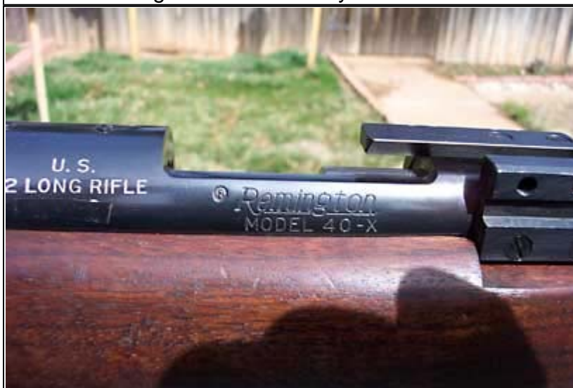
U.S. Stamp, Caliber Designation (Note aperture sight base and rear scope base)
