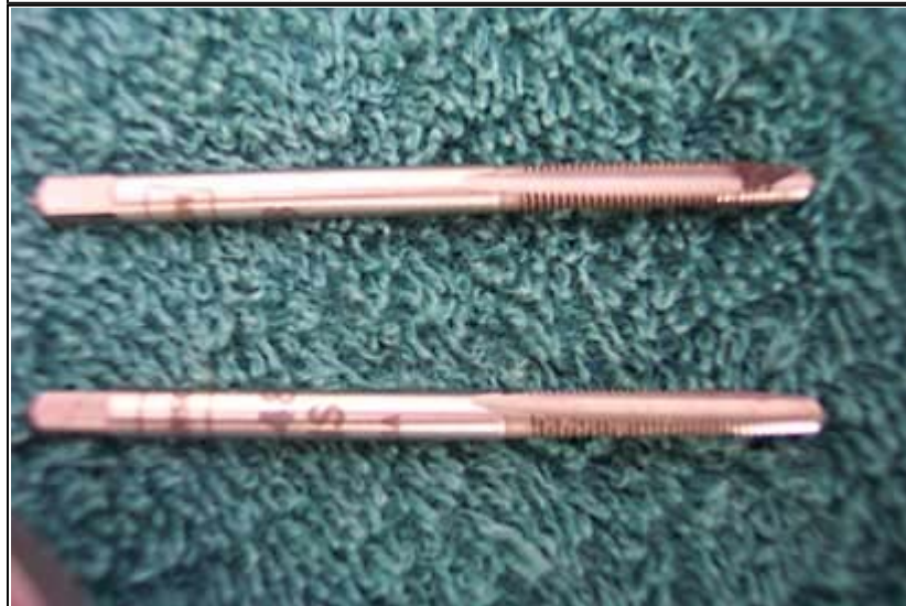
Bottom Tap Is Clean, Top Tap Cleaned Allot Of Dust And Old Oil From Threaded Holes!
