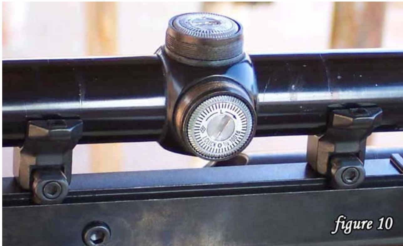
Eye relief and reticle set, bottom of scope rings moved to approximate centers of for and aft scope tube sections.
