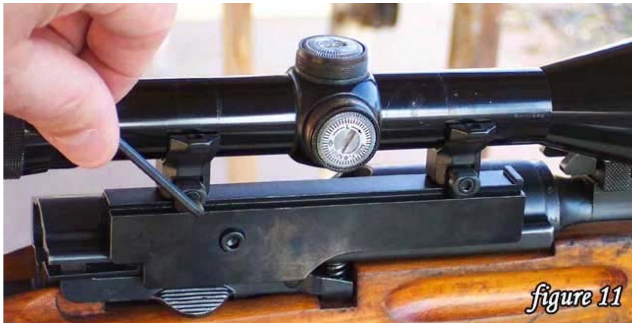
Locking bottom of scope rings to 3/8 dovetail
