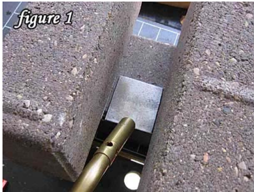
Metal test area was heated with propane torch for approximately 20 seconds. Bricks were placed on either side to control splattering.
