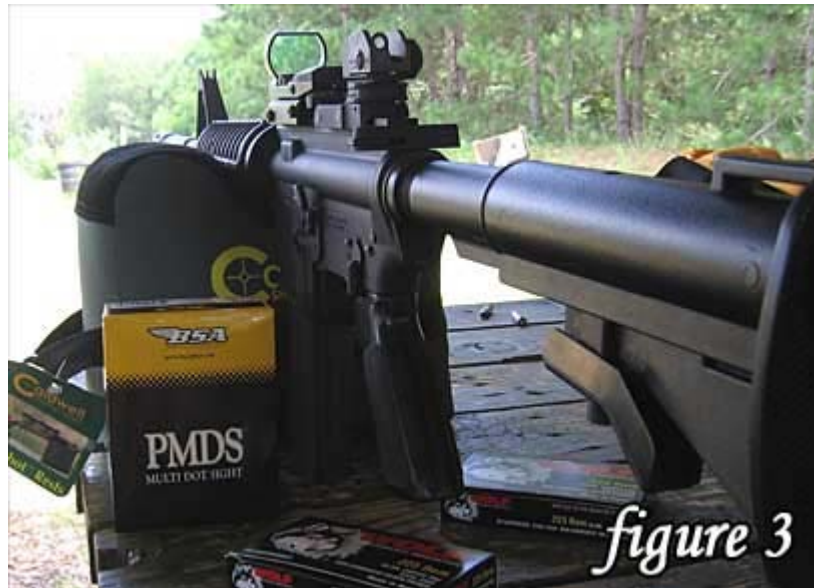
The BSA PMDS sight co witnesses nicely with the M4-clone flat top upper. The upper barrel/receiver and the rear A2 sights are DPMS. The lower is Stag Arms.
