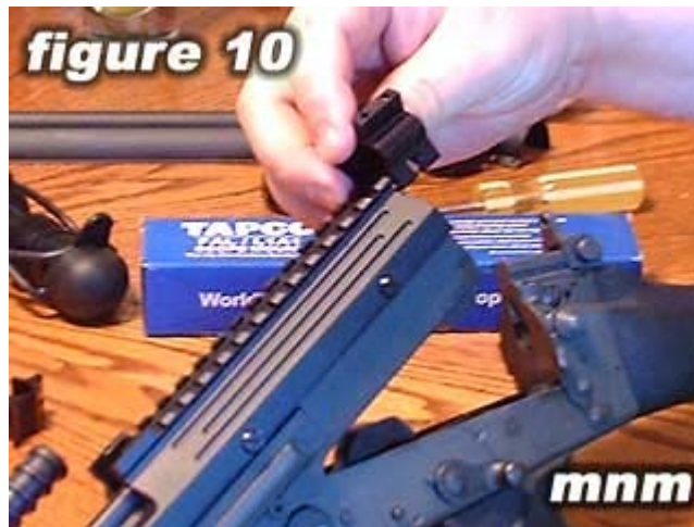
With the upper receiver open, slide the front scope ring into place.
