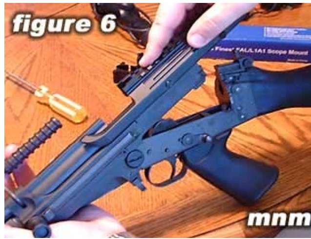
Slide the TAPCO receiver cover into place.
