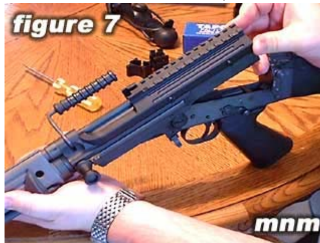
Push the scope mount receiver cover all the way forward.
