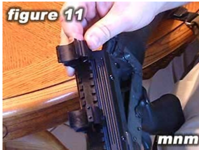
Next slide the rear scope ring into place.
