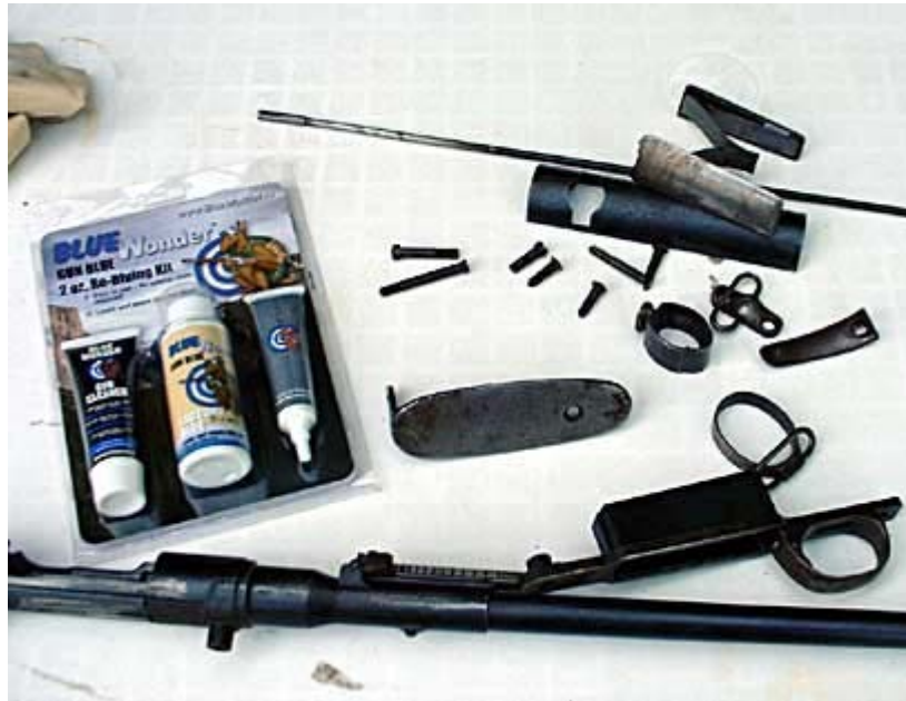
A VERY RUSTY ARISAKA TYPE 38. NOTE NON-EXISTENT BLUE ON SOME OF PARTS.
