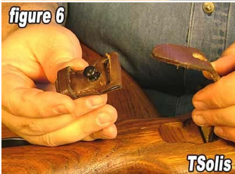
6) Figure 6 shows the keeper (Frosch) and the direction it should be installed.
