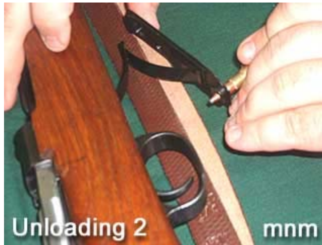
Release magazine door as shown in Unloading 2.
