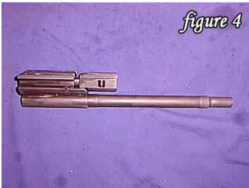
4) Full picture of the bolt body.
