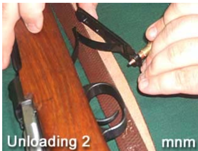
Release magazine door as shown in Unloading 2.
