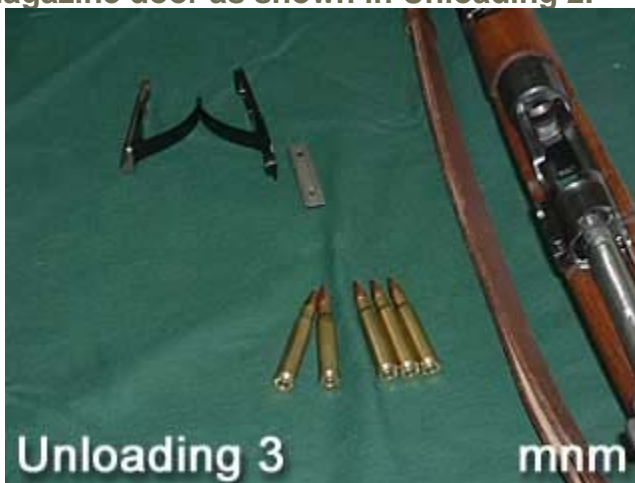
Allow all rounds in magazine to fall away from magazine. Safety Operations
