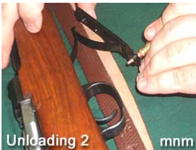
Release magazine door as shown in Unloading 2.
