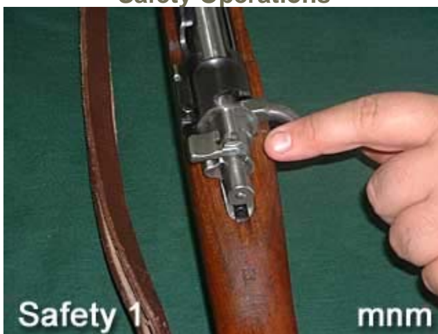
Safety 1 shows the Mauser safety in the off position.
