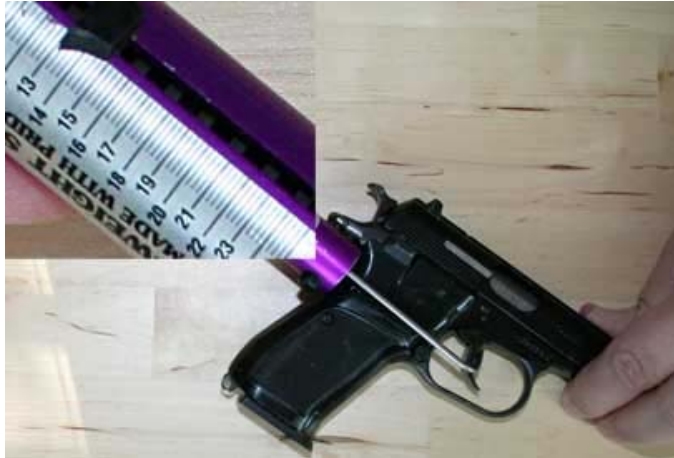
Double Action Trigger Pull at 13.25 Lbs.
