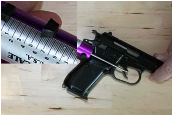
Single Action Trigger Pull at 5.75 Lbs.
