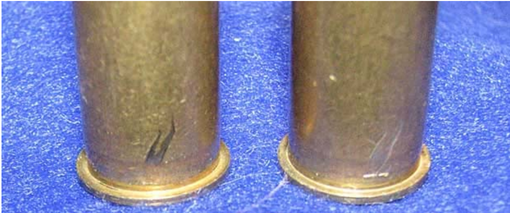
Figure 2 A close up view makes it easier to see where the burr is in the chamber. This is the area we will concentrate on. If the burr existed near the neck, the technique presented would not be used as it could very easily change shoulder/neck dimensions of the chamber.
