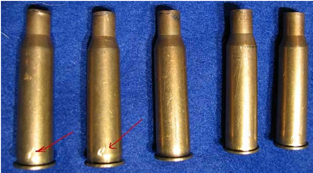
Figure 1 Marked in red are large gouges near the base of the brass case.
