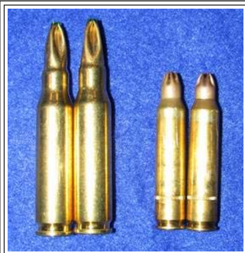
7.62mm on left, 5.56mm on right. Blanks can be denoted by the crimped ends in the case.
