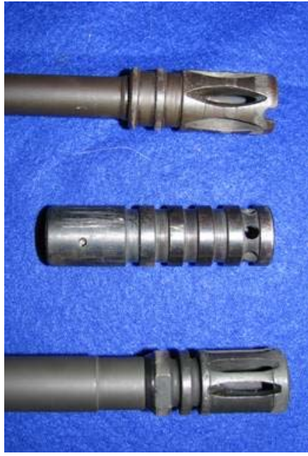
Some of the common types of NATO 22mm standard launchers include (top) FR 7/8, 59/66 SKS, and the AR's (A2 in this case)
