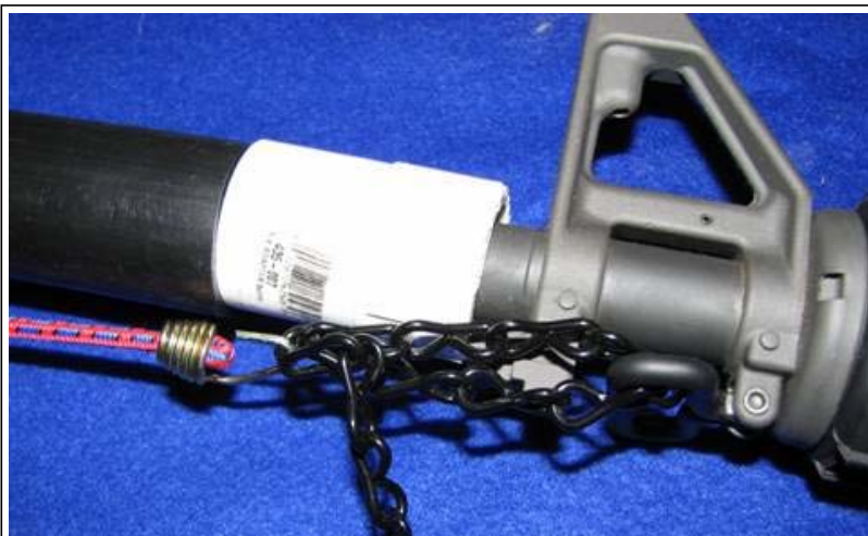
What I did was to slide a 1" long PVC union down the barrel first. Then I added a short piece of chain to extend the range of the bungee attachment.
