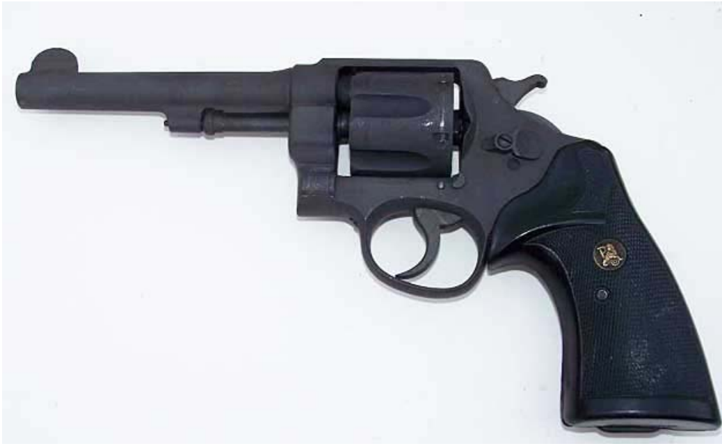
Figure 12 US 1917 with Pachmayer "Signature" grips (Notice lanyard ring showing at the bottom of the grips)
